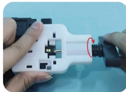
D Rotate the drill clockwise to drill out the chip.
